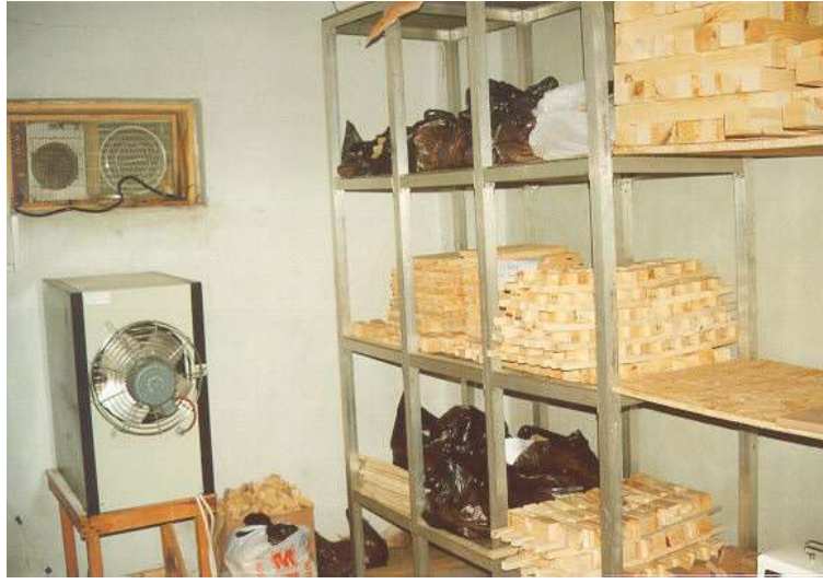
Şekil 2. Deney örneklerinin klimatize edilmesi Figure 2. Climatization of wood samples of the clones
